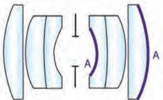
Figure 4: Conventional wisdom: asphere close to aperture stop and another close to image plane<sup>2</sup>
