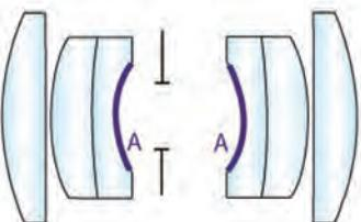
Figure 5: Aspheres surrounding aperture stop. Note the increase in airspace between aperture stop and aft optics<sup>3</sup>
