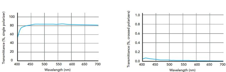
WGF (COP) Wire Grid Polarizing Film
