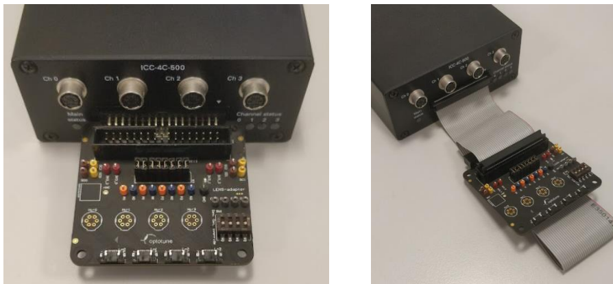
Figure 4: Adaptor board connection options
